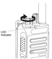
**NOTE:** The Home screen does not light up during a power up if the LED indicator is disabled (see *Turning the LED Indicator On or Off* on page 67).
