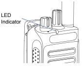
**NOTE:** The LED lights up solid green while the radio is transmitting and double blinks green when the radio is receiving a privacy-enabled call.
