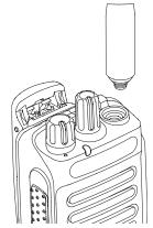
To remove the antenna, turn the antenna counterclockwise.
