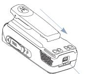
To remove the battery, turn the radio off. Move the battery latch into unlock position and hold, and slide the battery down and off the rails. Attaching the Antenna
